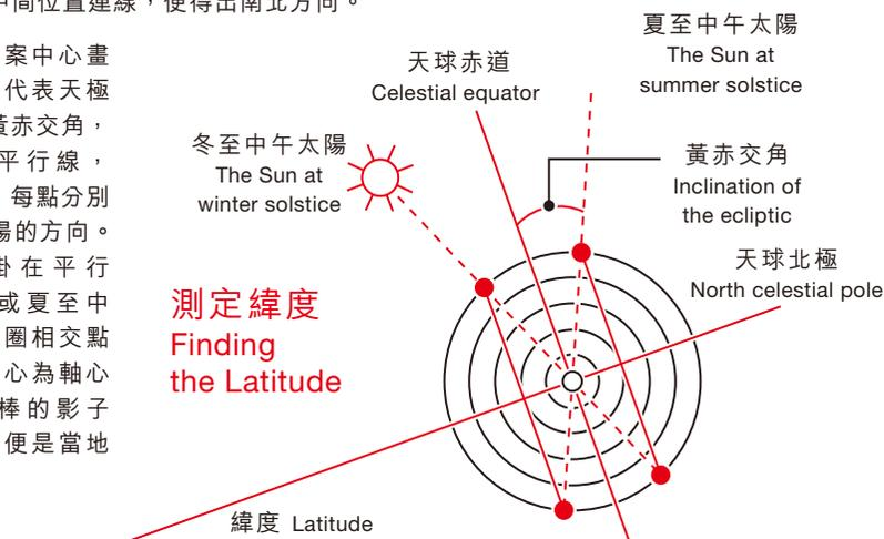
The direction determining table is an astronomical instrument designed by the astronomer *Guo Shoujing* of the *Yuan* Dynasty (1279-1368) to determine the direction and latitude.
