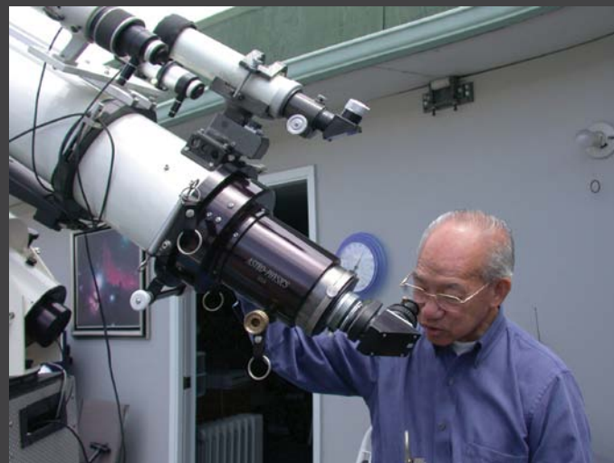
廖生正在檢查他的20.6cm折射鏡焦點，攝於2003年7月。廖生的觀測態度一向嚴謹，對焦時都十分認真。 Mr Liu is checking the back focus of his 20.6-cm refractor. He always demanded precise focusing during an observation. Photographed in July 2003.
