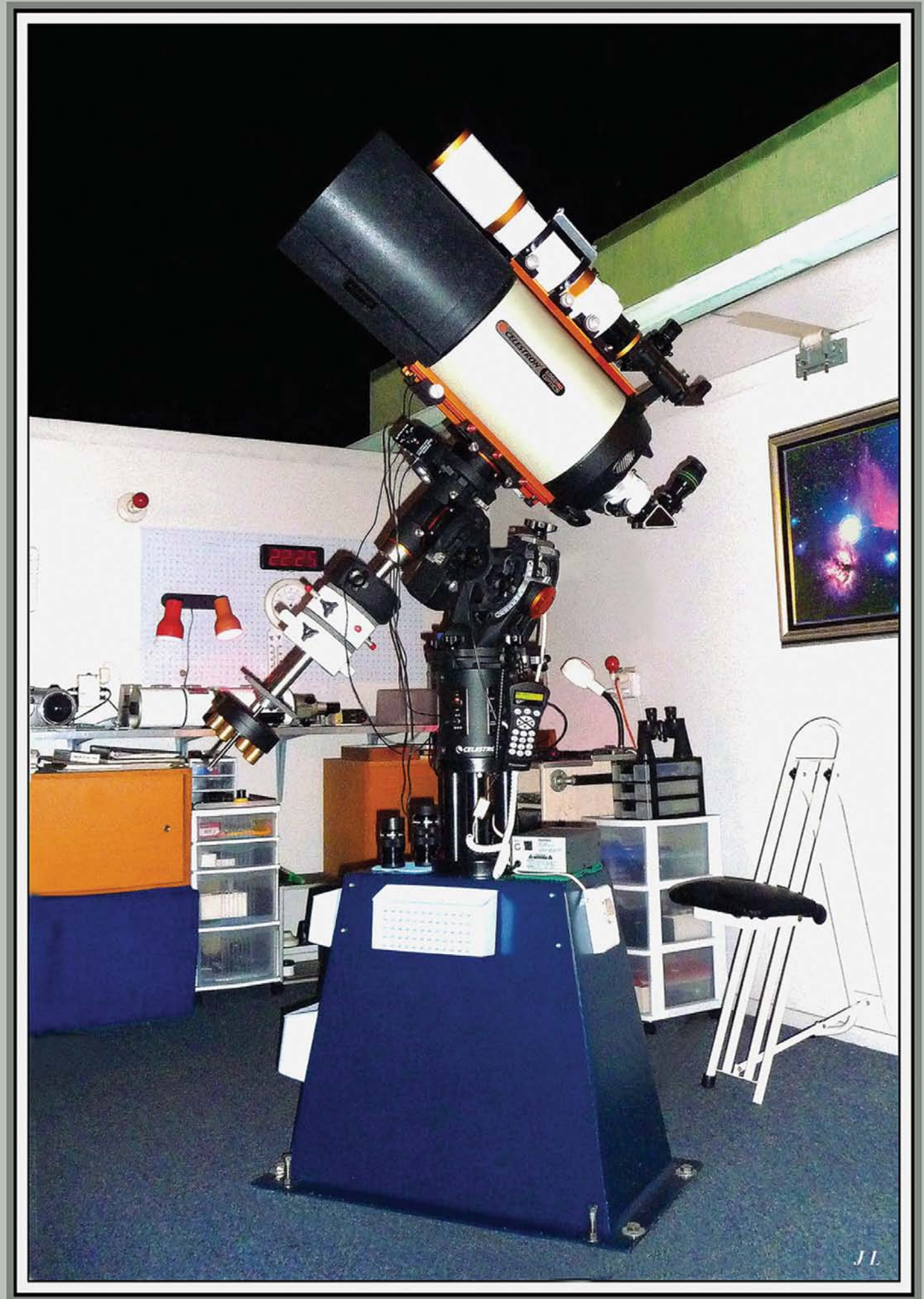
The new CELESTRON 28 cm f/10 Edge HD Schmidt - Cassegrain Telescope in my backyard.
