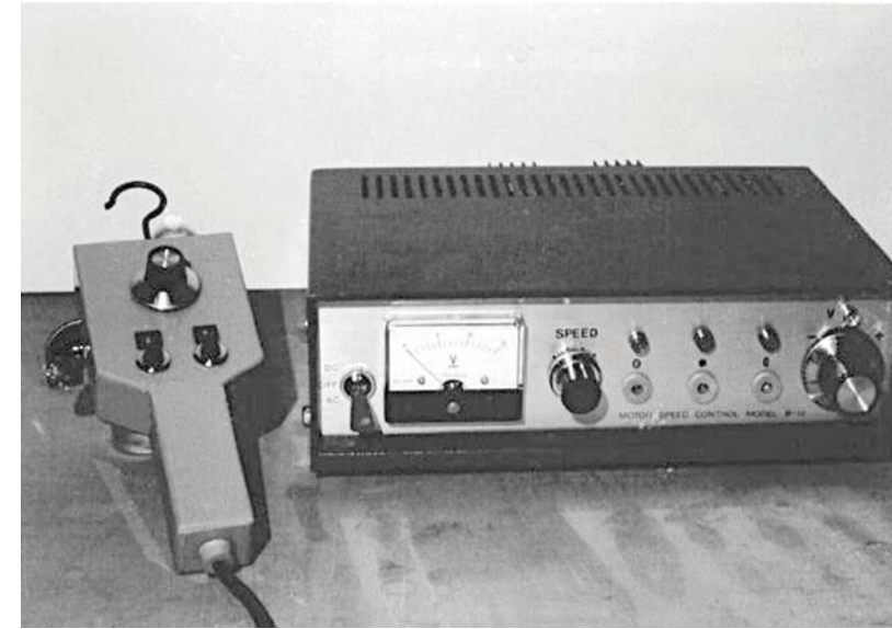
This electronic clockdrive, built by Chu for Joe in 1975, offers sidereal, lunar and solar tracking rates apart from the regular Fast / Slow buttons. Its short-term stability is ten-folds better than old designs which suffer from temperature drift.
