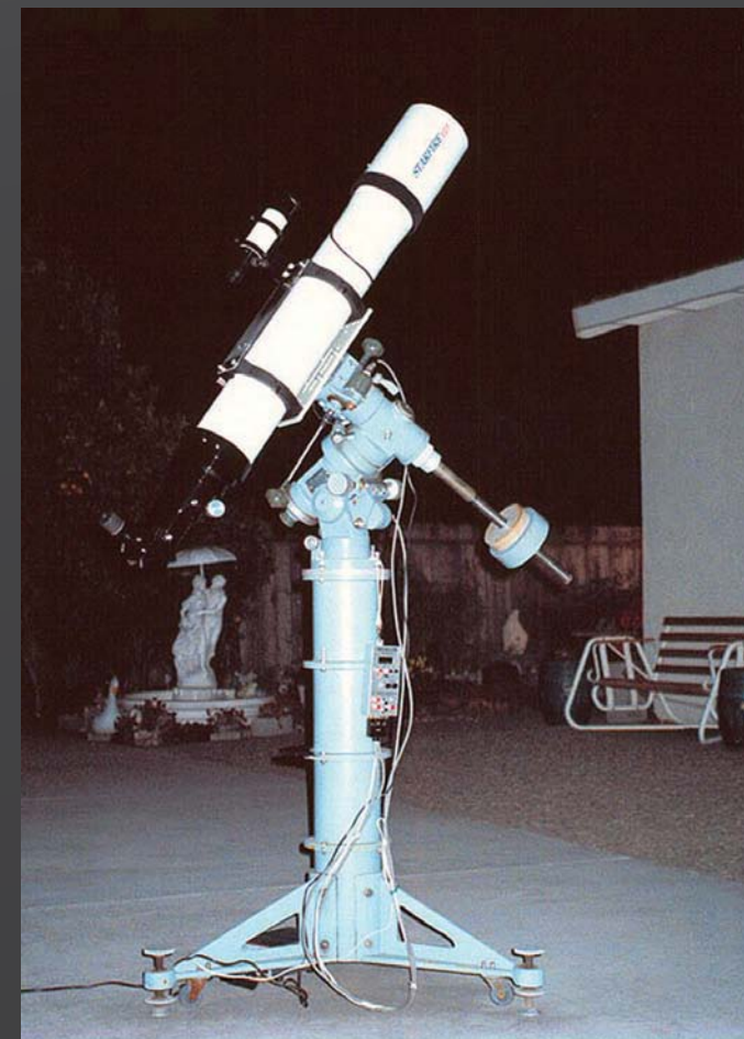
設在後院天文台外的13cm f/8 Astro-Physics EDT 折射鏡，以太陽觀測為主，也用於教育到訪的朋友及子女。 The 13-cm f/8 Astro-Physics EDT refractor outside the home backyard observatory, mainly for solar observation and sharing educational funs with visiting children and friends.
