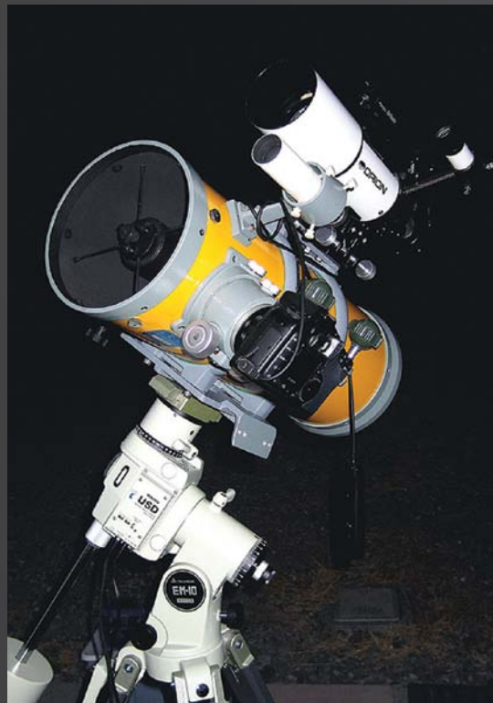
高橋Epsilon-160 f/3.3天文照相機和EM-10赤道儀，主鏡採用高精度的雙曲面，特大對焦器可容納直徑大至49 mm的影像。廖生在1980年購買此鏡，這一直都是他的戶外觀測至愛。 The Takahashi Epsilon-160 f/3.3 Astrograph on EM-10 mount. It employs a precise hyperboloidal primary mirror and an oversized focuser to allow an image circle as large as 49 mm. It was bought by Mr Liu in 1980 and was his outdoor favorite for a lifetime.
