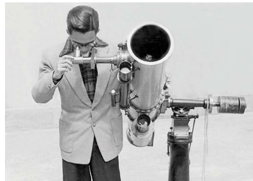
Joe and his second telescope — the Old Faithful 16.5cm (6.5inch) f/10 Newtonian reflector. It came with a gravity-driving clock to turn the gears of the equatorial mount, an illuminated finderscope and a micrometer for double star measurement. The picture was taken in 1953, Hong Kong.
